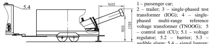
1 – passenger car; 2 - trailer; 3 - single-phased test transformer (IOG); 4 - singlephased multi-range reference voltage transformer (TNOOG); 5 - control unit (CU); 5.1 - voltage
