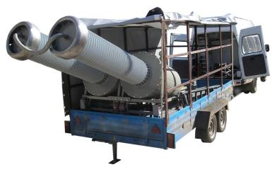
Gas-filled mobile metrological installation UMPG-330-I is designed for determination of errors of 35, 110, 220, 330 kV general-purpose voltage transformers directly at the site of their use.
